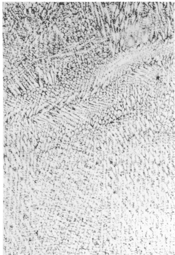
Figure 7 Typical metallographic structure of the surface-clad layers ( \times 50 ).
